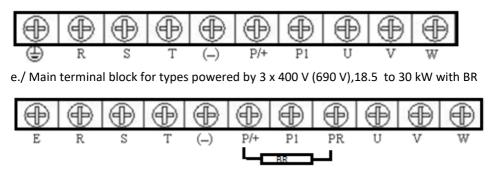
f./ Main terminal block for types powered by 3 x 400 V (690 V), 132 to 315kW
