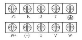
g./ Main terminal block for types powered by 3 x 400 V (690 V), 350kW and more.
