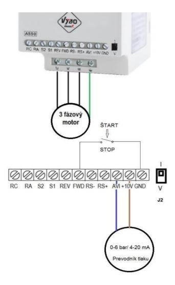
\* The wiring diagram applies only to a pressure transducer with an output of 4-20 mA
