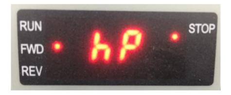
During PID operation (constant pressure control), you can use the up arrow (button) to add the desired set pressure, and conversely, use the down arrow (button) to decrease the value of the desired pressure even during operation.
