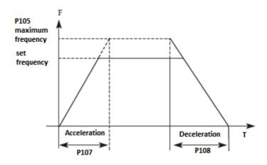
The preset deceleration / acceleration value is the primary time. Another deceleration / acceleration time can be selected by an external terminal.
