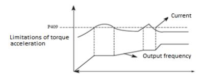
100% of the current is the rated current of the inverter; if P409 is set to 0 then the torque limitation is inactive and does not have a protective function.
