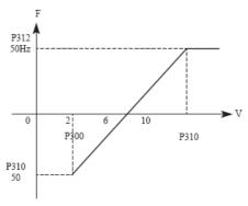
P300 = 2, minimum voltage input FIV: 2V (the inverter considers signals below 2 V for invalid signals);
