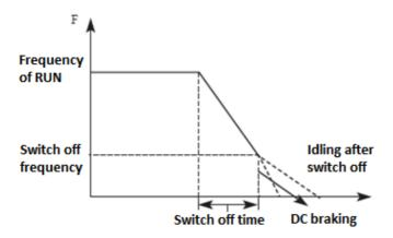
With regard to stop mode after reaching stop frequency, you can select the DC brake and other options. If you do not select DC braking, the engine will automatically stop in the idle mode.
