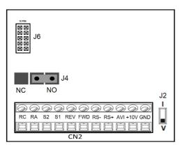
Switch J4 determines the logic of the output relay NO or NC.
