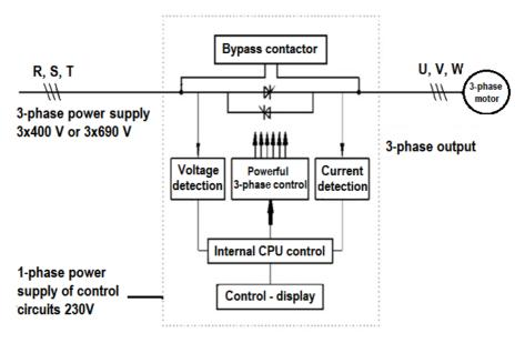
Figure 7.1 SSZ model
