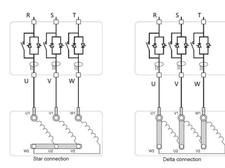
Connecting the electric motor
