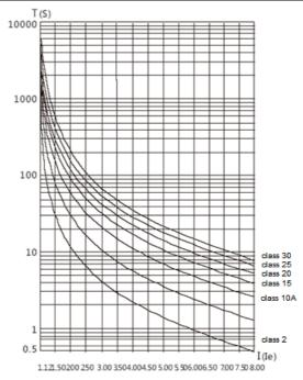
IEC609 74-4-2 Motor thermal protection curve
