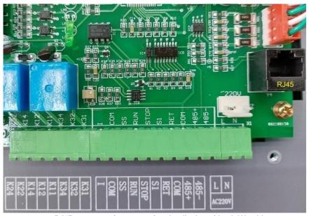
RJ45 connector for connecting the display with a LAN cable
