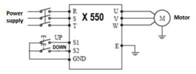
Parameter: P317 = 15, terminal S1 will be set in UP mode P318 = 16, terminal S2 will be set in DOWN mode.
