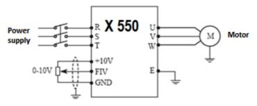
Explanation: the control output frequency of the inverter is controlled by the AI / FIV voltage signal from the external POT (10 k $\Omega$ ).
