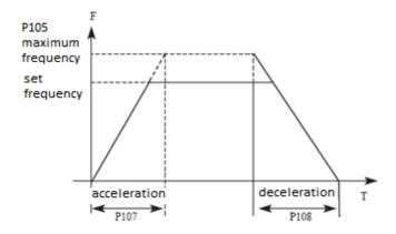
The default deceleration/acceleration value is primary time. A different deceleration / acceleration time can be selected via an external terminal.
