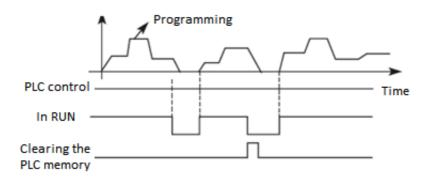
During the running of the PLC program, due to a fault or stop, the frequency inverter will automatically record the program status, after removing the fault and turning on the inverter again, the frequency inverter will continue to operate according to the program. If memory clearing is enabled, the program will be reset and the drive will start from the beginning.
