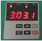
If you set P000=07, the display of the X550 inverter shows the PID setting
