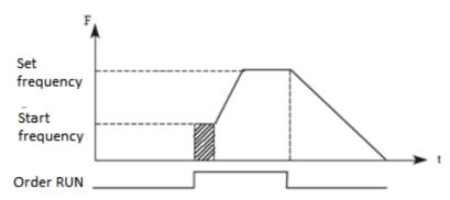
The starting frequency is the initial frequency at the start of the inverter. For equipment with heavy load or fast fast torque, it increases the starting frequency. However, if the trigger frequency is too high, it may cause the over-protection to activate.
