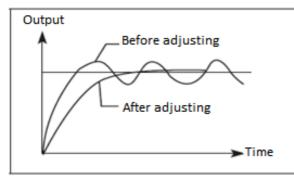
Limitation of the system outlet during oscillation a: decrease the differential time (D value) or set to 0 b: decrease the proportional constant (P)
