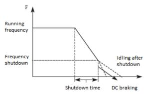
As for the stop mode after reaching the stop frequency, you can choose DC brake and other options. If you do not select DC braking, the motor will automatically stop in coasting mode. 1: Idle to stop
