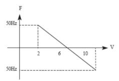
Example 2, the output from the control PC is 4 - 20 mA and the inverter has the "Output frequency" parameter set: 100 Hz - 0 Hz
