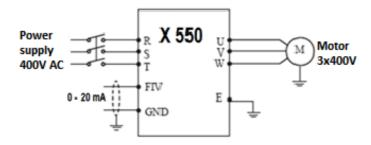
Explanation: the control output frequency of the inverter is controlled by the AI / FIV current signal 0 to 20 mA, or 4 to 20 mA.
