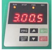
The "SLP" display has changed to "3.0 0.5" the inverter display shows the value of the required pressure 3.0 bar on the left and the pressure value in the system on the right, i.e. 0.5 bar. The inverter has been activated and the pump motor starts to reach the required pressure of 3.0 bar.
