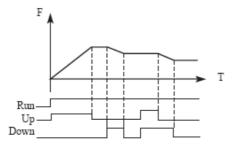
Explanation: if UP is active (UP is closed), the frequency will increase. If DOWN is active (DOWN is closed), the frequency will decrease.
