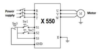
Use S1, S2 or S3 as input terminal for external signal
