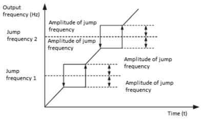
Figure 4-12: The principle of jump frequencies and amplitude
