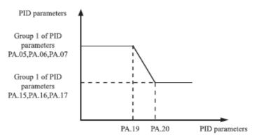
Figure 4-24 Switching PID parameters
