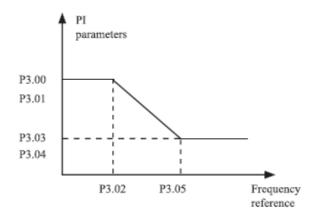
Figure 4-4: The relationship between running frequency and PI parameters
