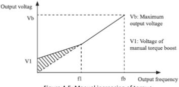
Figure 4-5: Manual increasing of torque
