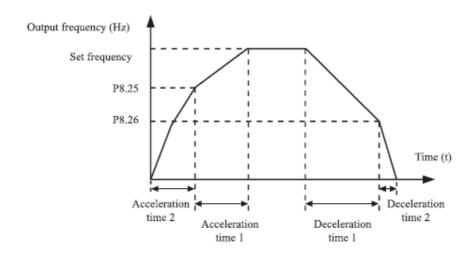
Figure 4-17: Toggle acceleration / deceleration time
