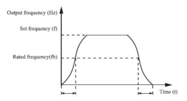
Figure 4-1 S-curve acceleration / deceleration B
