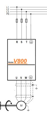
P0.00= 2 P0.01= 0 P0.08= 120 sec P0.09= 120 sec P1.10= 1 P2.01=7,5 kW P2.02= 400 V P2.03= 13,5 A P2.04= 50 Hz P2.05= 2930 rpm P4.01= 5,0 % P9.00= 1 P9.01= 10 P9.03= 50 P9.12= 11 P9.13= 1 START
