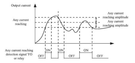
Figure 4-21 Detecting any current
