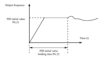
Figure 4-25 Functions of initial value the PID
