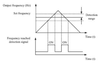
Figure 4-15 Frequency detection range
