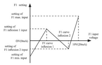
Figure 4-29 Diagram of curves 4 and 5
