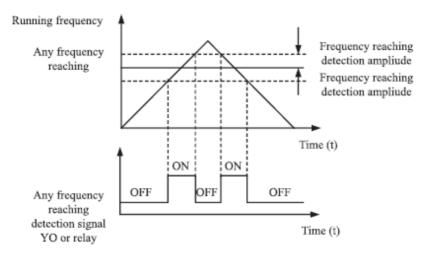
Figure 4-18: Detection of any frequency
