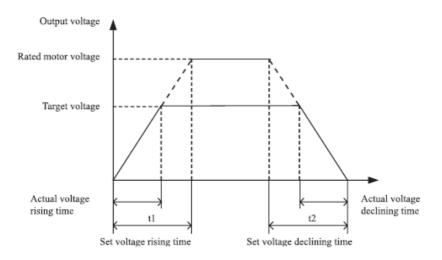
Figure 4-7: Voltage course at V/F separation
