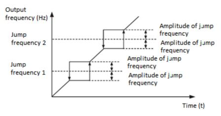
Figure 4-16: Diagram when the jumping frequency is enabled during the acceleration / deceleration process
