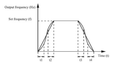
Figure 4-2 S-curve acceleration / deceleration A
