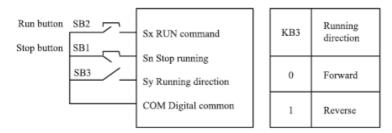
Figure 4-10-2: Setting the three-wire mode 2
